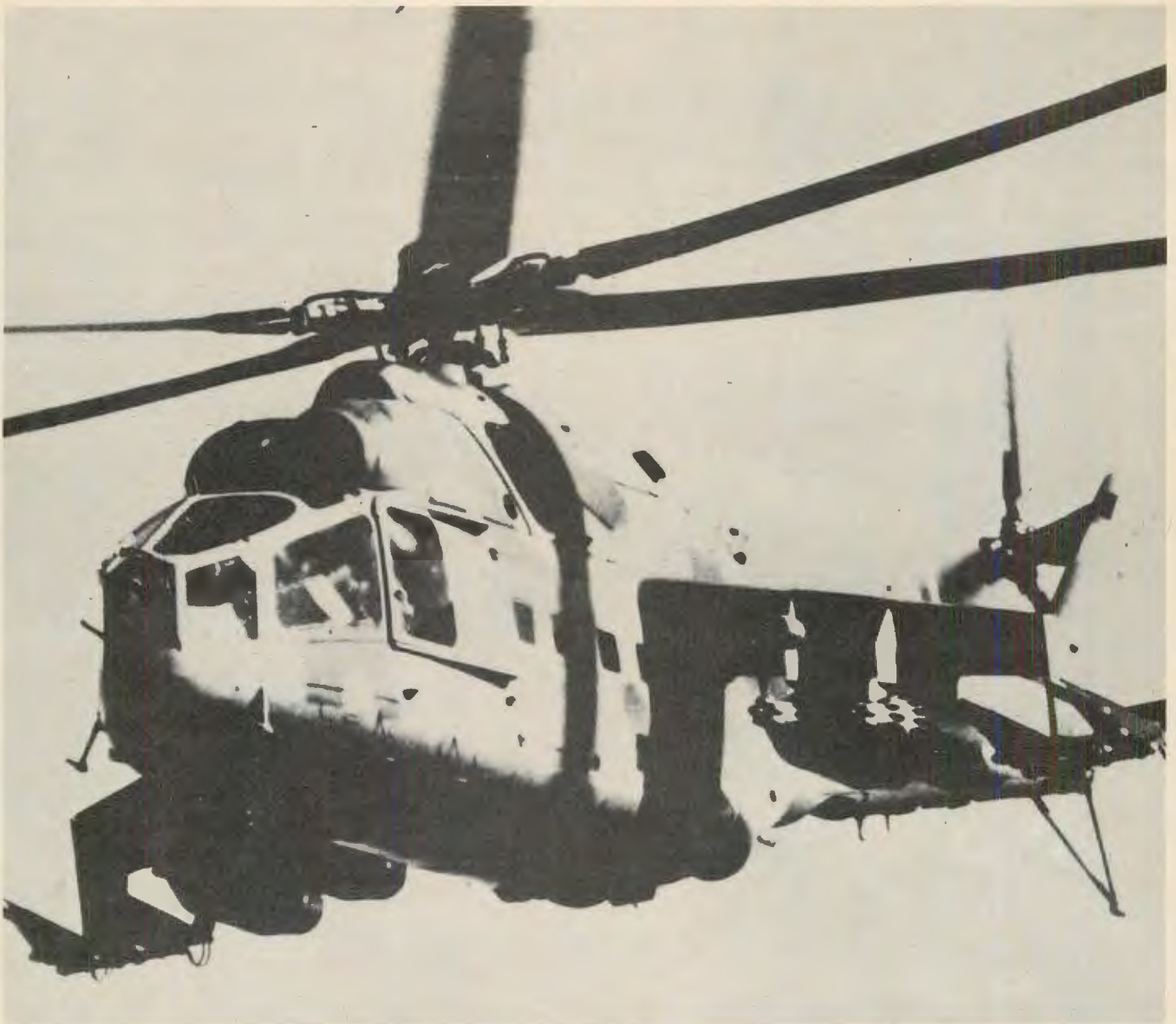
Mi-24 "Hind-A" attack helicopter. These heavily armed aircraft and newer "Hind-Ds" play important role in Soviet unconventional operations and have been heavily used in Afghanistan. "Hind-As" use 12.7mm machine gun under the nose and 57mm rocket pods, mounted on stub wings, against soft targets, and can carry up to four "Swatter" or "Sagger" ATGMs. Cabin, aft of cockpit, accommodates eight to 16 troops. Small-scale operations will probably use "Hinds" to provide fire support and carry troops. Photo: U.S. Army
